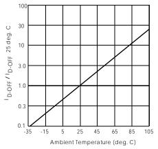
Figure 5. Typical Normalized Off-State Leakage
