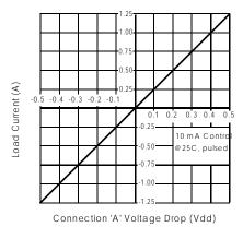
Figure 3. Linearity Characteristics
