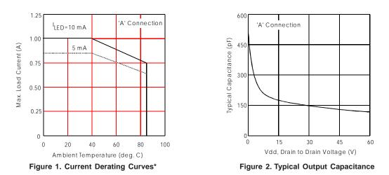
\* Derating of 'B' and 'C' connection at +85°C will be 70% of that specified at +40°C and is linear from +40°C to +85°C.
