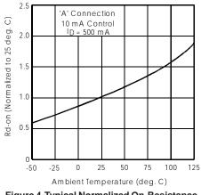
Figure 4. Typical Normalized On-Resistance
