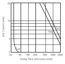
Figure 7. Typical Delay Times
