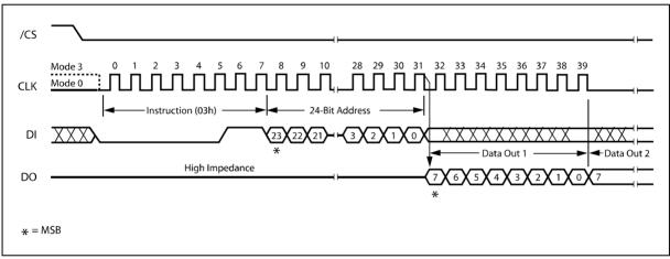
Figure 8. Read Data Instruction Sequence Diagram
