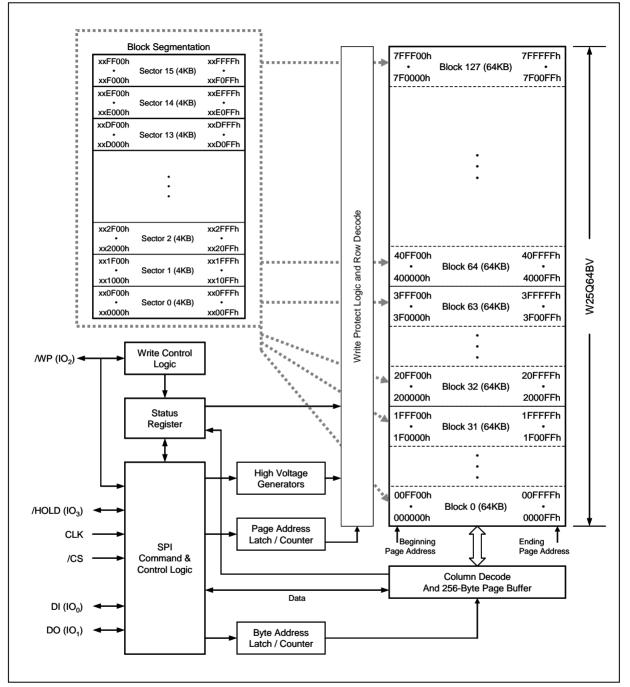
Figure 2. W25Q64BV Serial Flash Memory Block Diagram
