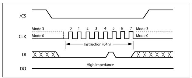
Figure 5. Write Disable Instruction Sequence Diagram
