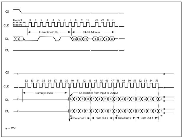
Figure 10. Fast Read Dual Output Instruction Sequence Diagram
