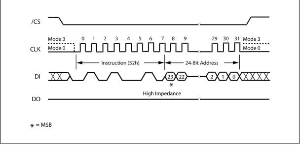
Figure 18. 32KB Block Erase Instruction Sequence Diagram
