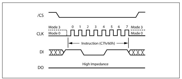
Figure 20. Chip Erase Instruction Sequence Diagram
