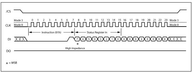
Figure 7. Write Status Register Instruction Sequence Diagram
