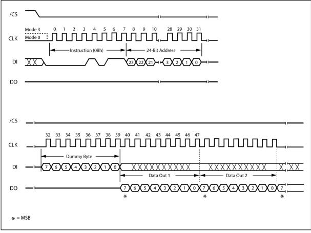
Figure 9. Fast Read Instruction Sequence Diagram
