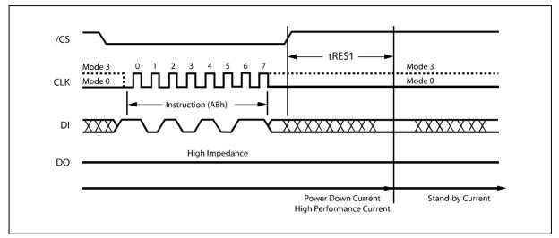
Figure 25. Release Power-down/High Performance Mode Instruction Sequence
