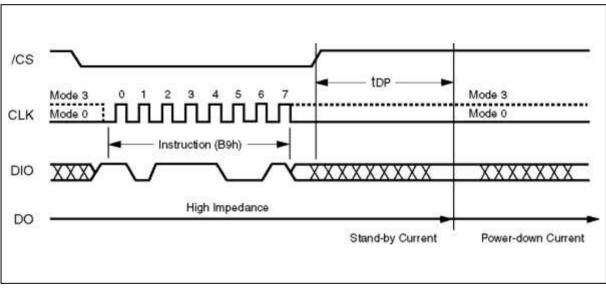
Figure 23. Deep Power-down Instruction Sequence Diagram
