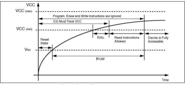
Figure 31. Power-up Timing and Voltage Levels
