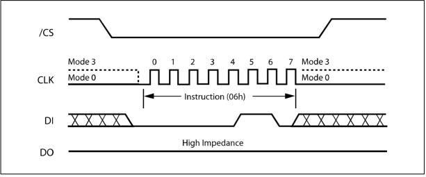
Figure 4. Write Enable Instruction Sequence Diagram
