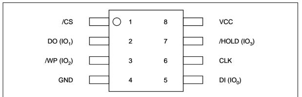
Figure 1a. W25Q64BV Pin Assignments, 8-pin SOIC 208-mil (Package Code SS)
