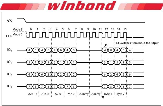
Figure 13b. Fast Read Quad Input/Output Instruction Sequence Diagram (M7-0 = Axh)
